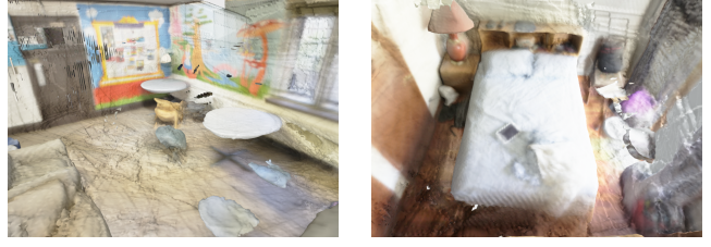
Figure 6. With scale calibration and volumetric fusion, room-scale geometry initialization can be achieved from monocular depth without any optimization of the voxel grid parameters. The remaining task would be refining noisy regions and prune outliers.
